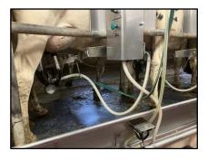
We also check for unit alignment and hose length. Pictured at left, too long of hoses leads to more vacuum fluctuation at the teat end. When we are finished doing our vacuum measurements, we graph all of the pulsators.
